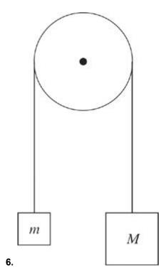
Assuming a frictionless, massless pulley, determine the acceleration of the blocks once they are released from rest.
